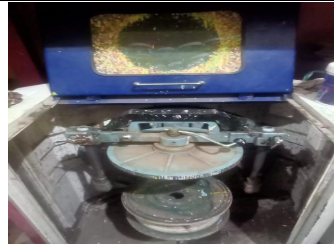
Figure 6: Gyro shaker is used to mix the solvent with colorants within 2-5 min
