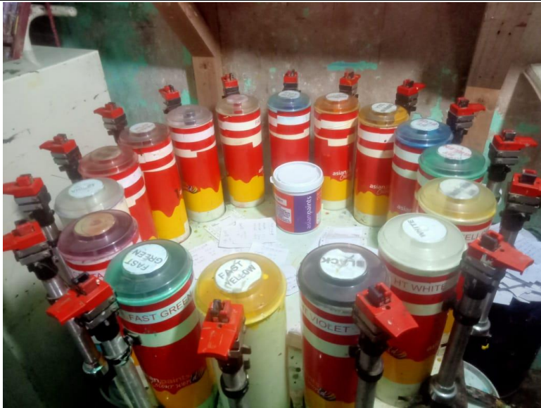
Figure 5: Asian Paints manual tinting machine with 16 colorant slots
